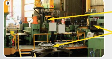
The forming station is a helical 3 roll bending theory with a 200 ton press used to form coils with a thicknesses of up to 1". This particular station can form coil into pipe up to 10' 7" diameters
