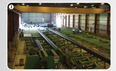
We have 3 pipe repair stations where we complete welds due to machine stop/starts and also complete the skelp weld on the outside of the pipe and make any other repairs identified by UT and visual inspection.
