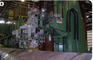
We can apply ultrasonic testing to 100% of our welds with our inline ultrasonic testing machine. We can then mark any defects to inspect and repair after the pipe gets cut to length and moved off the mill.
