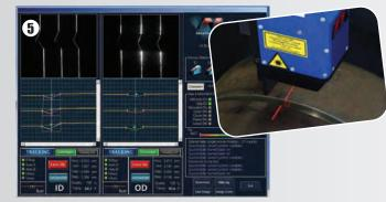
Weld groove center alignment is ensured by an automated laser tracking system.
