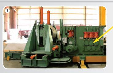
Once the coil is inserted into the machine, it advances with the first set of drive rollers through the five roll flattening stage to prepare the coil for edge milling and forming.
